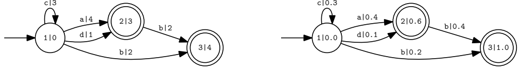
(a) An example of DPFA, state \lambda and transitions leading to it are omitted (b) Corresponding DPFA with probabilities
